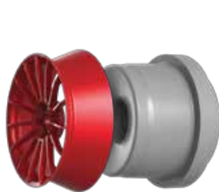
Cast blank placed into FlowForm mold
