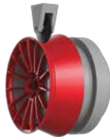
Roller presses onto blank and begins to mold wheel
